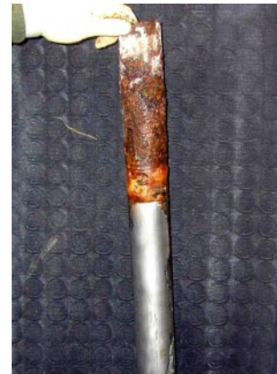
(Left) Insulated pipes in a 5% aerated salt bath. (Center) Same pipes 365 days into test. (Right) Pipe inspection after 365 days in salt solution. No corrosion in surface conversion treated areas.
