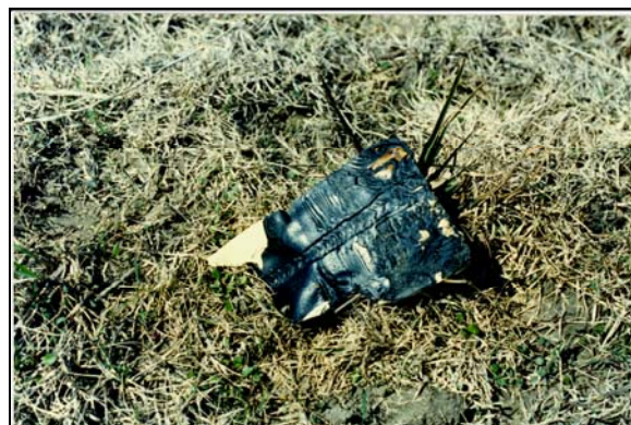
This photo illustrates how the corrosion control coating used in 606 Filler Tape conforms and fills voids.
