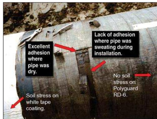
RD-6 applied for three years on partially sweating pipe in severe soil stress area. No bond to area where pipe was sweating at installation, but pH was 11 on water under the coating proving “Fail Safe”. Notice wrinkles on white tape, but no wrinkles on RD-6.
