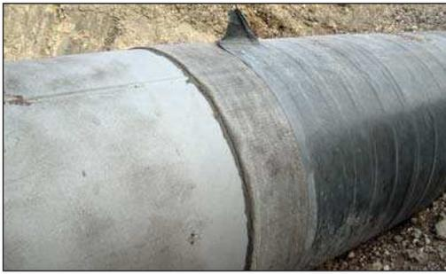
RD-6 coating system condition shown is after one year in severe soil stress area. Use of "Slip Plane" non-shielding, non-bonded outer wrap enhances soil stress resistance.
