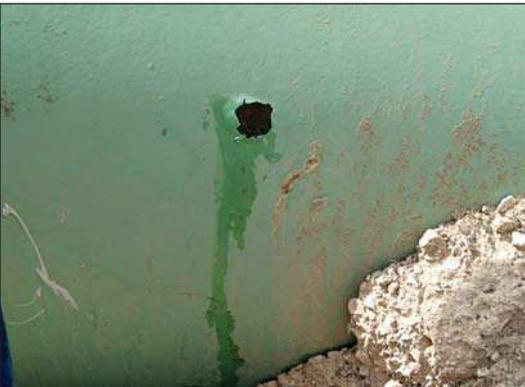
“Fail Safe” FBE coating in central U.S. with blisters. Water pH was 12 with no corrosion under FBE.
