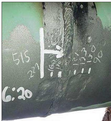
Soil stress caused wrinkles in shrink sleeve on 10-inch pipe which allowed water and SS shielded CP, resulting in significant corrosion after eight years.
