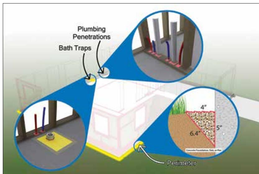
Polyguard’s TERM product line can be used in three key areas serviced by PMPs. TERM Particle Barrier is applied in a small trench around the perimeter of the structure and TERM Bath Trap Barrier is applied around plumbing penetrations and bath traps to prevent pest access.
