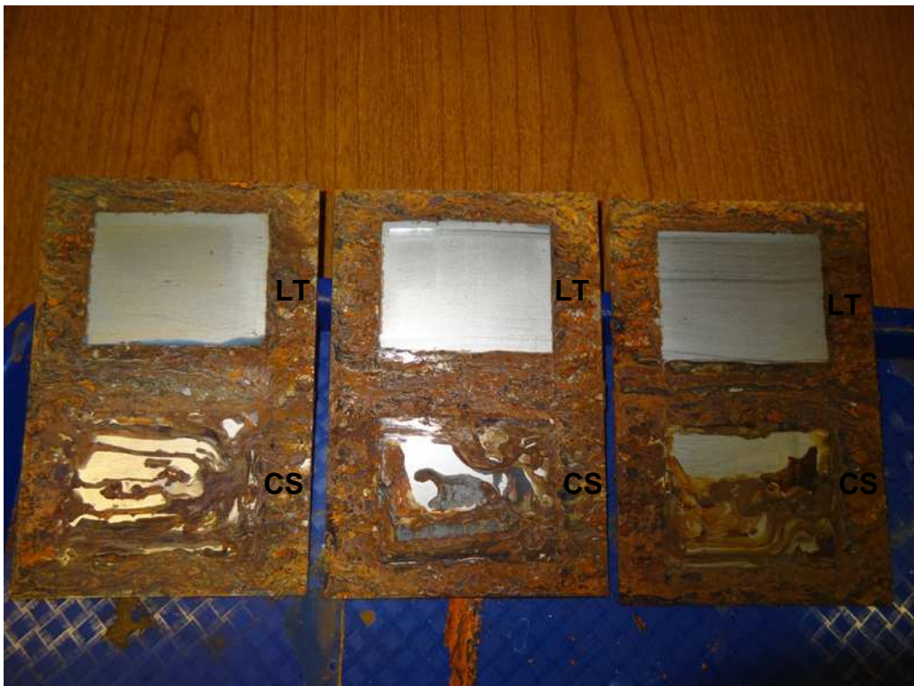
168 Hour Salt Spray Test Panels, Post Exposure - After Removing Coatings from the CRS Panels
