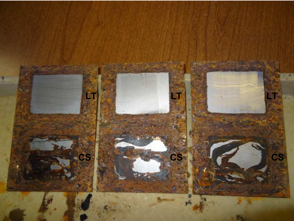
504 Hour Salt Spray Test Panels, Post Exposure - After Removing Coatings from the CRS Panels
