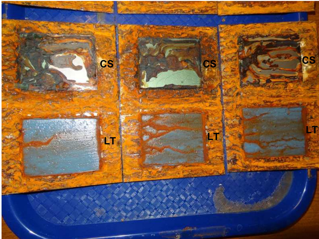
168 Hour Salt Spray Test Panels, Post Exposure
