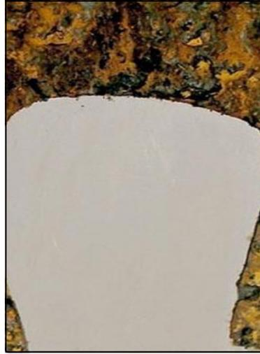
ASTM B-117 Salt fog testing was done to demonstrate **RG-2401's** corrosion stopping ability. The gel was applied to a blasted steel panel and subjected to 2000 hours in the salt fog test. When removed from the test (*left photo*) corrosion rates were aggressive. After cleaning the panel (*right photo*) the metal was as "shiny new" as before testing. Note the defined edges - **NO UNDERCUTTING**.
